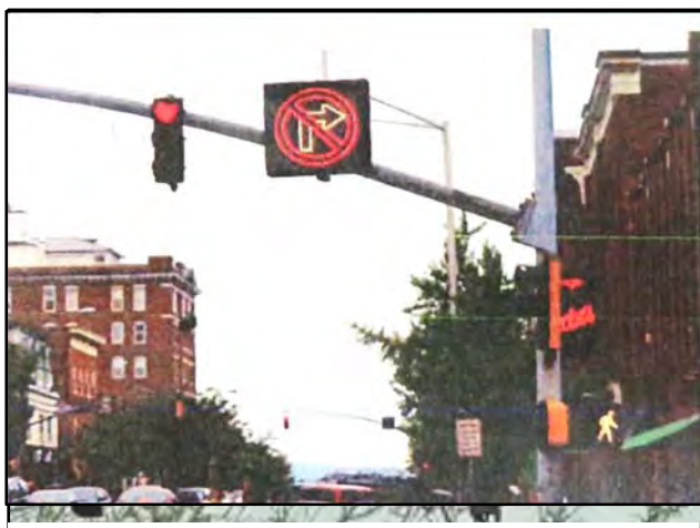
Figure 31: Leading pedestrian interval with no turn on red dynamic sign. (Source: Presentation: 2009 MUTCD New Provisions for Pedestrians and Bicyclists , John LaPlante & Richard Moeur)
